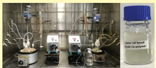
Lab Scale Reaction Setup to synthesize the Castor Oil based Acrylic Co-polymer
