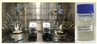
Lab Scale Reaction Setup to synthesize the Castor Oil based Acrylic Co-polymer
